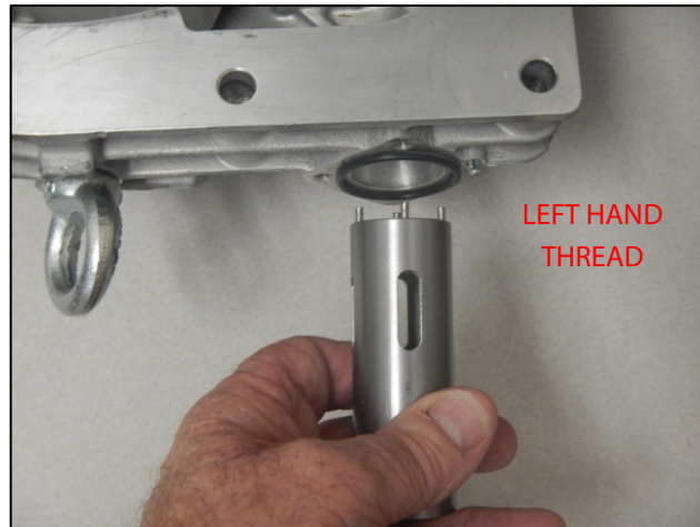
Figure 2. Locking Collar Tool Usage
