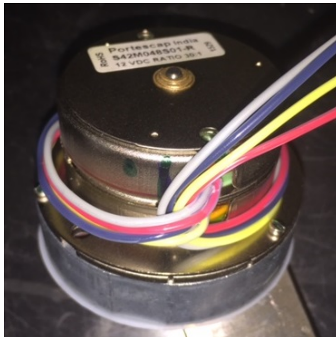
Figure 5 – IGV Motor Wiring
