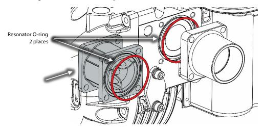
4. Finger-tighten the four provided M10x30 fasteners to secure the Resonator to the Compressor housing. Do not tighten at this time.
